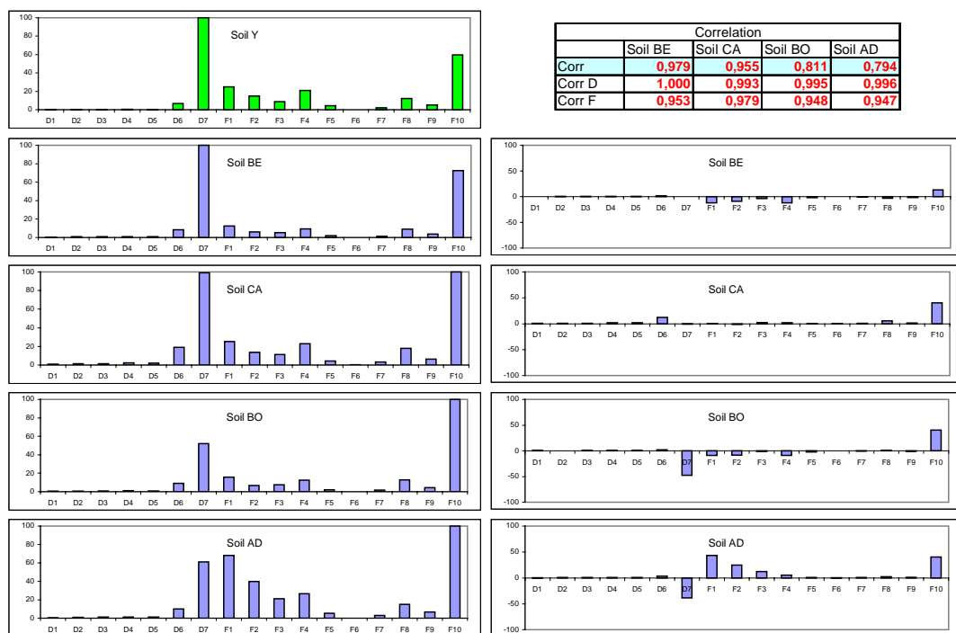
Figure 2: PCDD+PCDF profiles of the five soil samples. In the table are reported the Pearson correlation coefficients for the dioxins (Corr.D) and for the furans (Corr.F), calculated with respect to profile of the Y sample. In the left side are shown the profiles of the five samples, in the right side are shown the profile differences among each profile and the Y sample, the lowest contaminated one.
